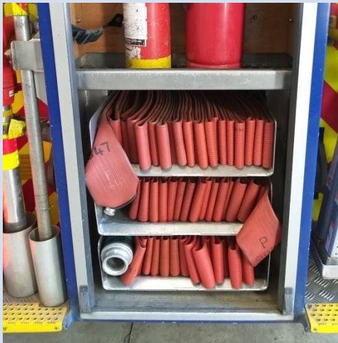
Sample feeder, 6 lengths (30m x 90mm) stowage on current Type 3, in rear locker.
