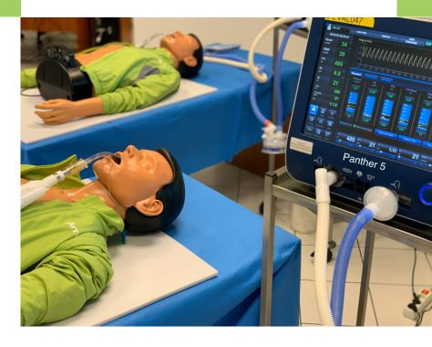
The **Panther 5 Ventilator** is an ICU level ventilator utilizing response to patient demand and very fast and stable pressurization during pressure breaths.
